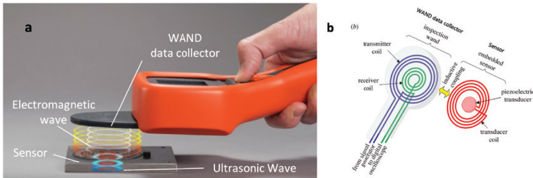
Figure 1. (a) Operation of WAND system, and (b) details of the inductive coupling between the WAND data collector and ultrasonic thickness sensor.
