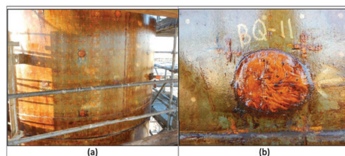
Figure 5. Photographs of sensors after months in service on a “live” plant. (a) Overview of installed sensors and measurement grid with fixed WT probe visible. (b) Detail of sensor BQ11 showing high levels of couplant and poor surface state.
