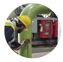
Thanks to ECHO extension coil, thickness measurement locations that were previously hard to reach could be accessed easily
