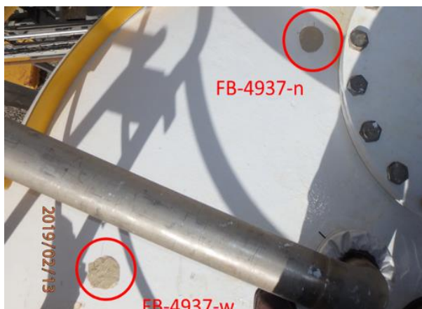
Examples of sensors installed on the tank head and connected pipework
