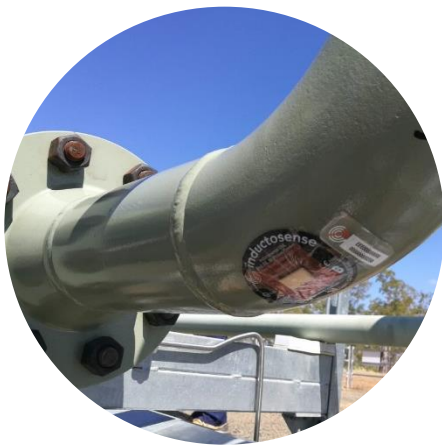
WAND sensors installed at sand erosion examination points (prior to coating)
