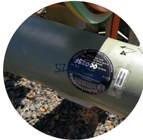
WAND sensors installed at sand erosion examination points (prior to coating)
