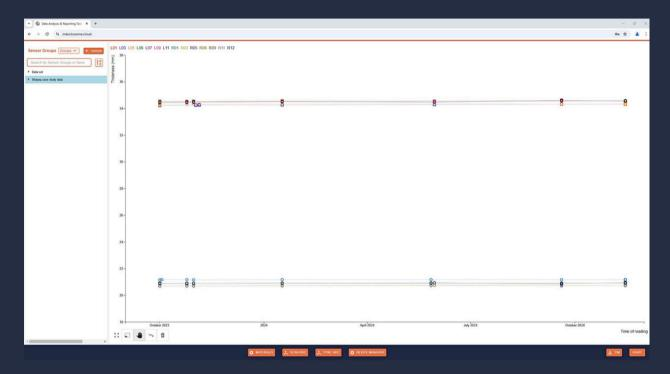
• The iDART software enables analysis of the ultrasonic A-scan before and after application of the Stopaq WrappingBand over top of the sensor.
