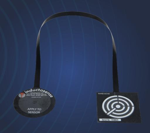
The Inductosense ECHO is an extension coil designed to work with WAND TM Sensors. One end of the coil is applied over a pre-installed sensor (over the sensor coating), and the other end becomes the new data collection location. The ECHO is ideal for difficult-access locations such as underneath insulation, confined access, or at height.
