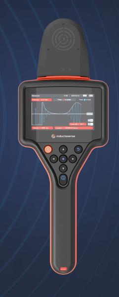
An easy-to-use handheld device that wirelessly activates and collects a thickness reading from a WAND TM Sensor when in close proximity. The interface displays the wall thickness, A-scan and sensor location information. The HDC is designed so that anyone can take an ultrasonic thickness measurement in the field, with the simple press of a button.
