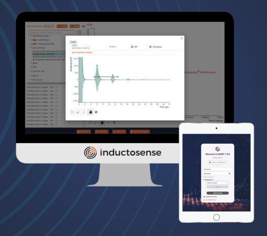
Inductosense Data Analysis and Reporting Toolkit (iDART) is a cloud-based software package for use with the Inductosense WAND system. iDART is available as both a desktop based and browser-based package, and enables configuration of your WAND devices, as well as management and analysis of your WAND thickness data.
