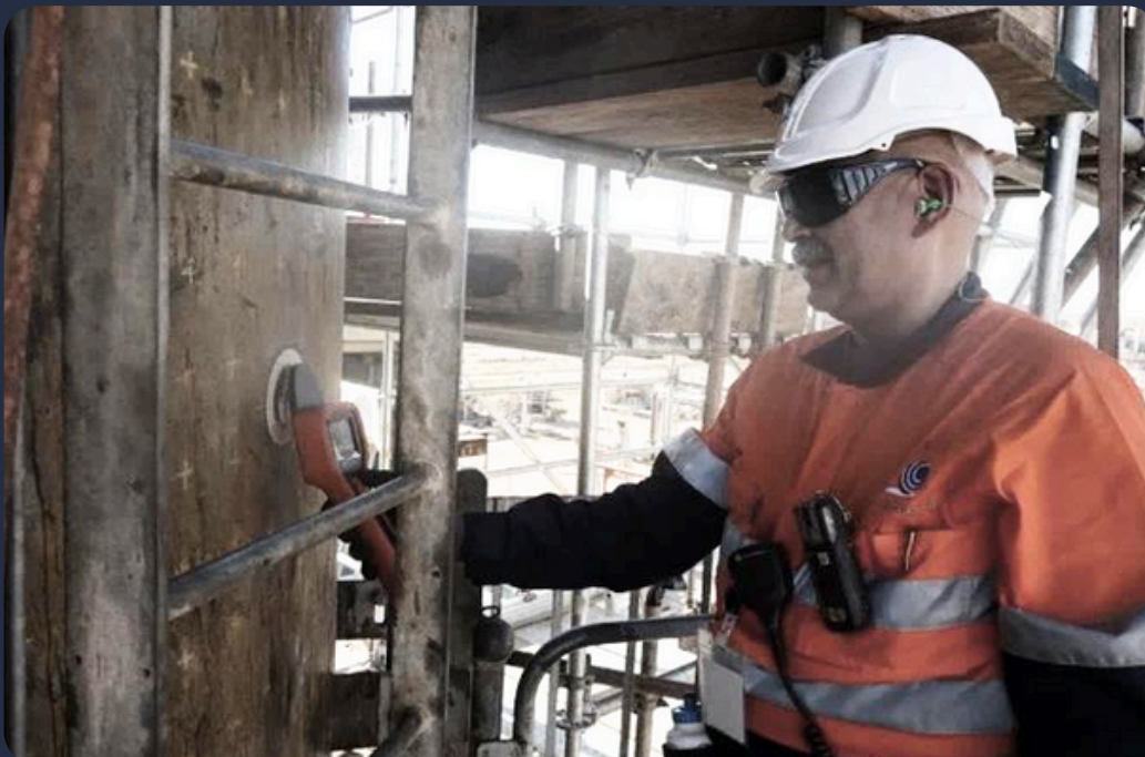
Onsite personnel were able to easily acquire thickness readings, without needing to prepare the surface each time.
