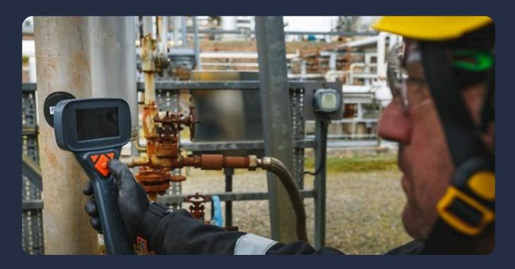
Thickness data from the permanently installed sensors acquired quickly and easily using the WAND handheld data collector.
