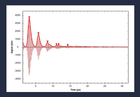
Example A-scan from one of the WAND sensors installed on the customer's pipeline, as shown in Inductosense's Data Analysis & Reporting Toolkit.
