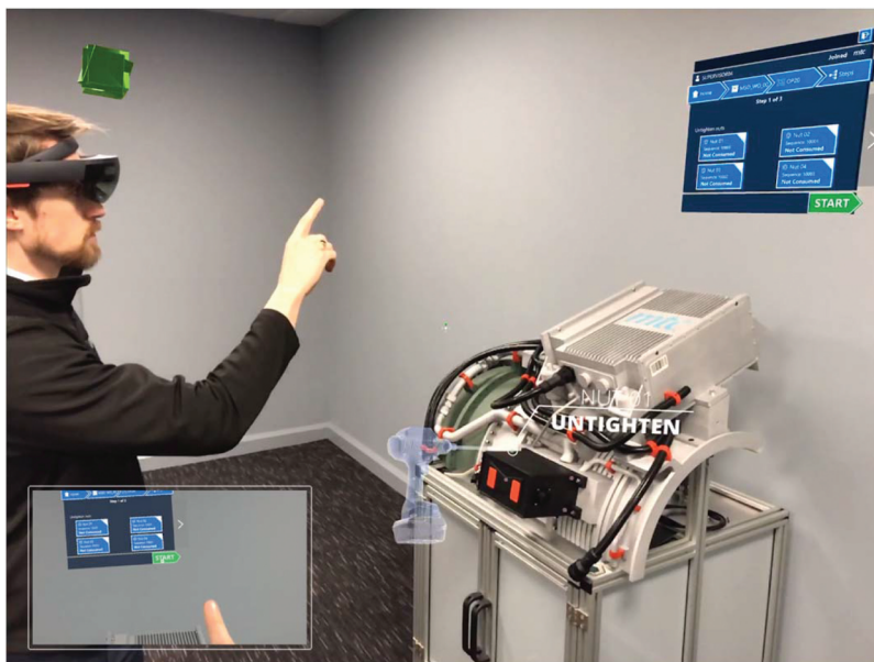
Figure 5. Screen capture from a cooperative demonstration of AR for a maintenance task. The “supervisor’s” view is shown. This consists of the current scene with current instruction overlays and process menu generated for the “operator”. A section of the “operator’s view” is also provided as an inset, related to the selected “operator” as marked by the floating geometric icon.
