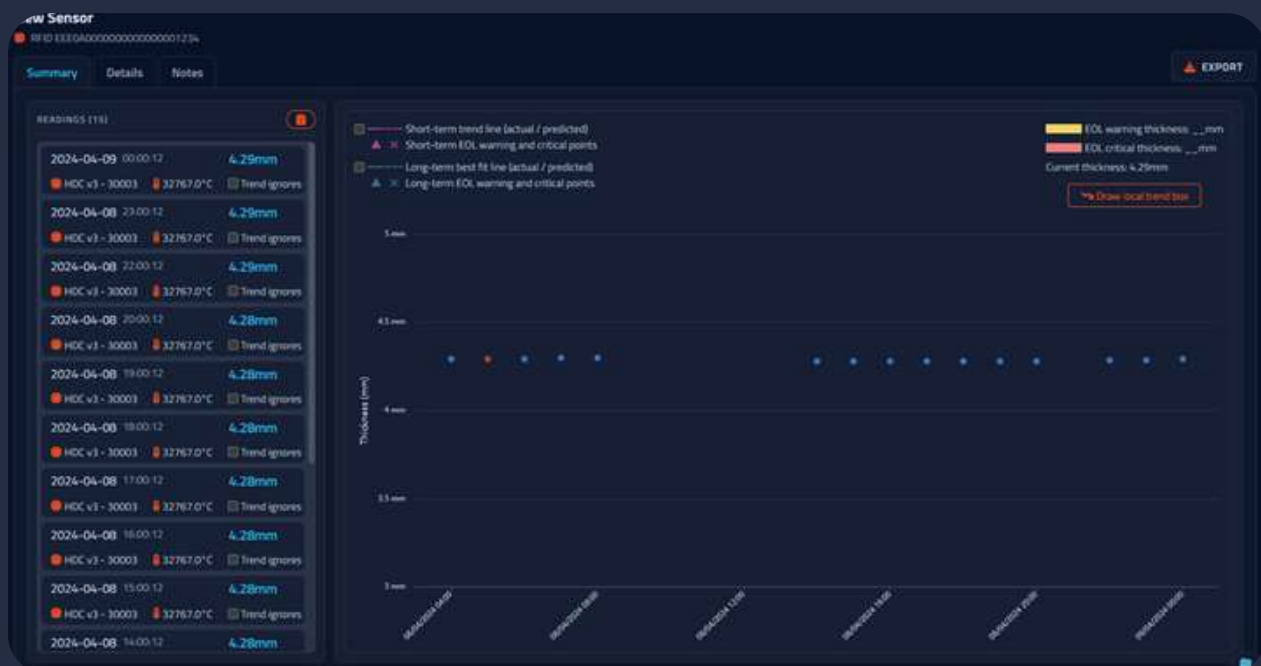
Figure 3: Thickness data from multiple installed WAND TM Sensors using iDART
