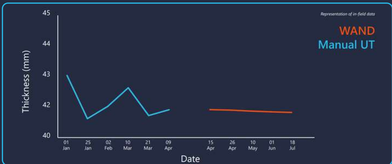
Figure 6: Transition from manual UT measurements to the WAND solution
