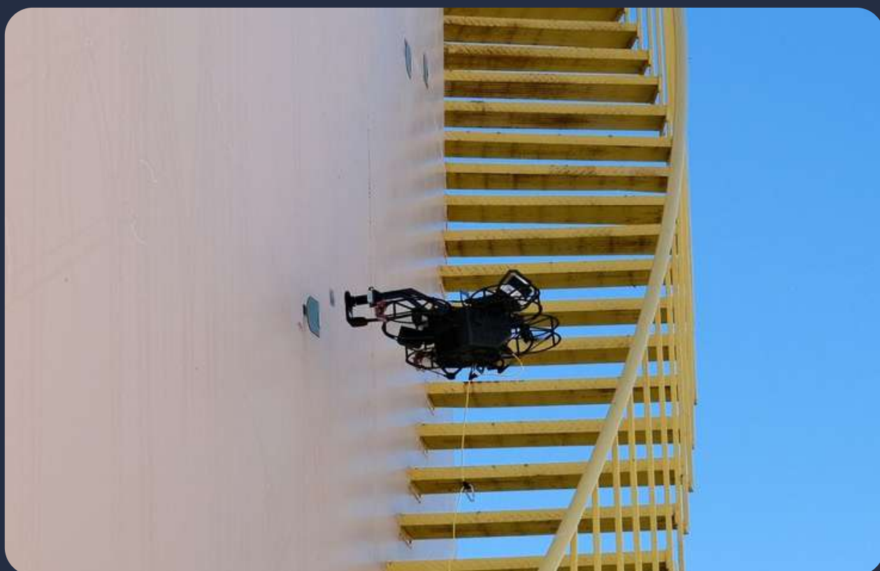
Figure 5: Example of WAND-PDC data collection using the Scout 137 Gen
