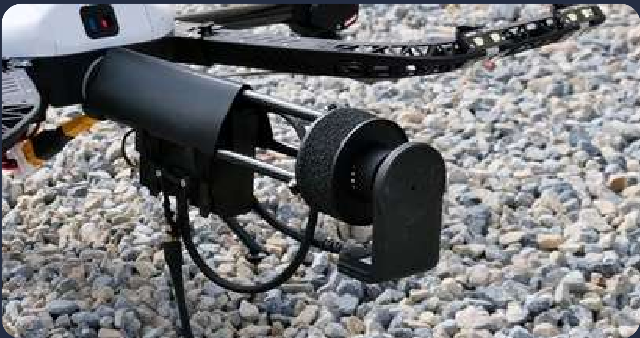
Figure 2: WAND-PDC attached to a Voliro T drone
