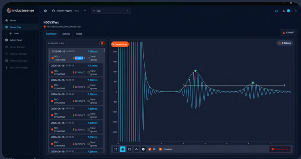
Figure 4: Ultrasonic A-scan analysis from a WAND TM Sensor using iDART
