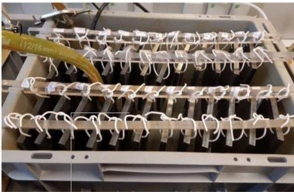
Coupons in the tidal corrosion test rig
