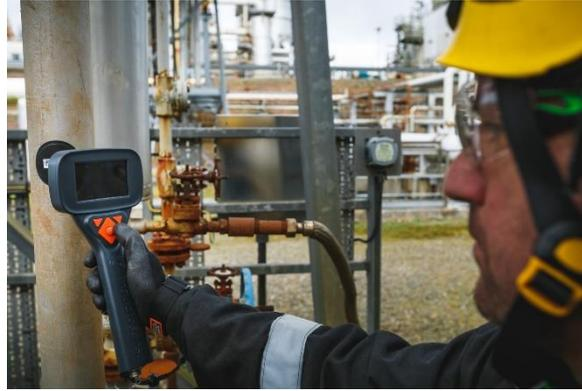
Thickness data from the permanently installed sensors acquired quickly and easily using the WAND handheld data collector
