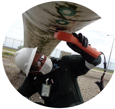
Accurate internal corrosion rate trending capability using the permanently installed WAND sensors
