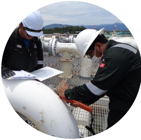
Thickness readings were collected and logged quickly and conveniently using the WAND data collector
